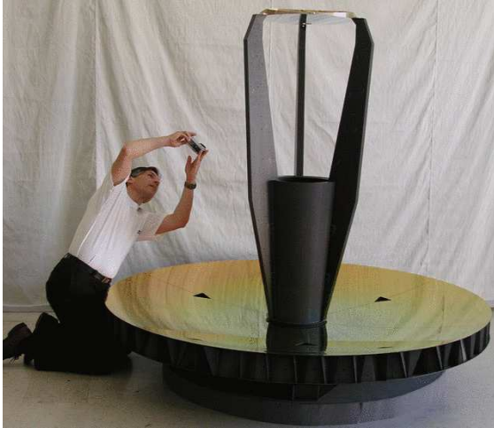
Figure 2.16.1: The COI mirror assembly
