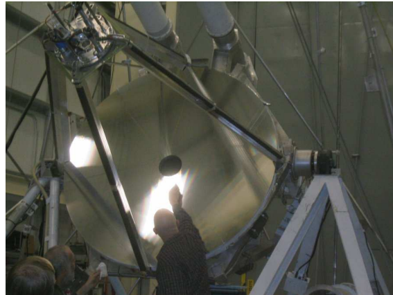
Figure 2.16.2: The Bosma mirror assembly for BLAST06 , including the recut primary, the 0CTE carbon fibre struts and Active Focus Mechanism.
