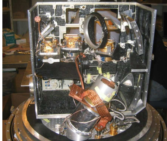
Figure 2.21: The BLAST optics box sitting on the cold plate. Two faces of the box have been removed to allow access. Light from the Cassegrain telescope enters through the window at bottom left. M3 is at bottom right, M5 at top right. The cylindrical M4 is at centre, attached to a copper heat strap. The ring at top centre holds one of the dichroic beam splitting filters (not installed). The second filter ring is also missing, but would be attached just to the left of the one present. From left are the 500\ \mu\text{m} , 350\ \mu\text{m} , and 250\ \mu\text{m} bolometric arrays. Attached to the cold plate in front of the optics box, bottom centre, is the ^3\text{He} fridge.
